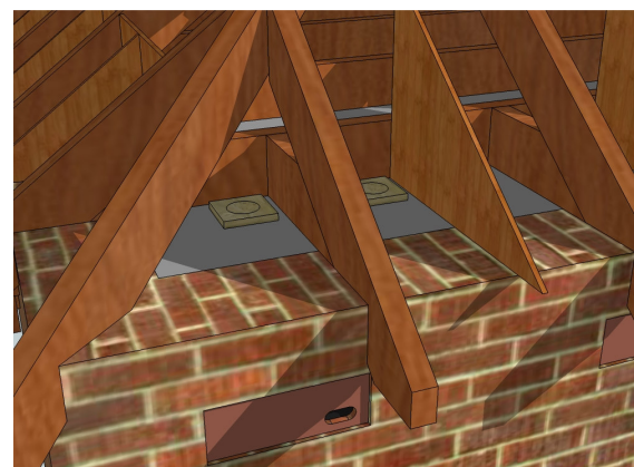
Diagram showing an Ibstock style brick and boxed joists for open eave access with artificial swift nest platforms in place.
