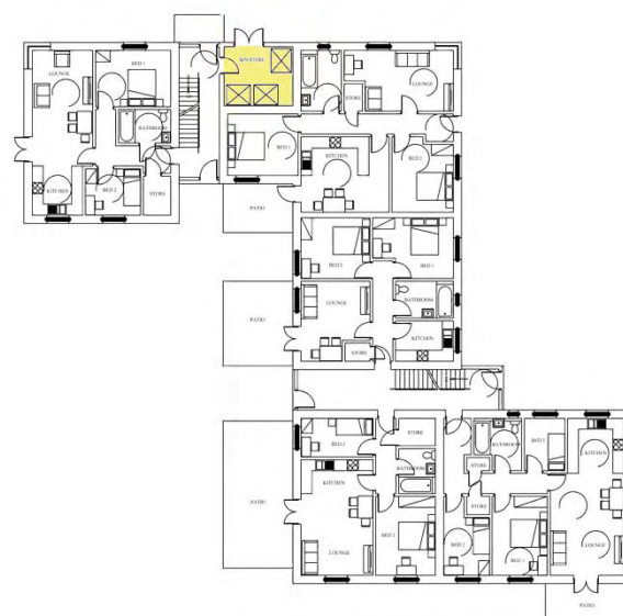
Figure 8.7 An example of bin store incorporated into the building design
