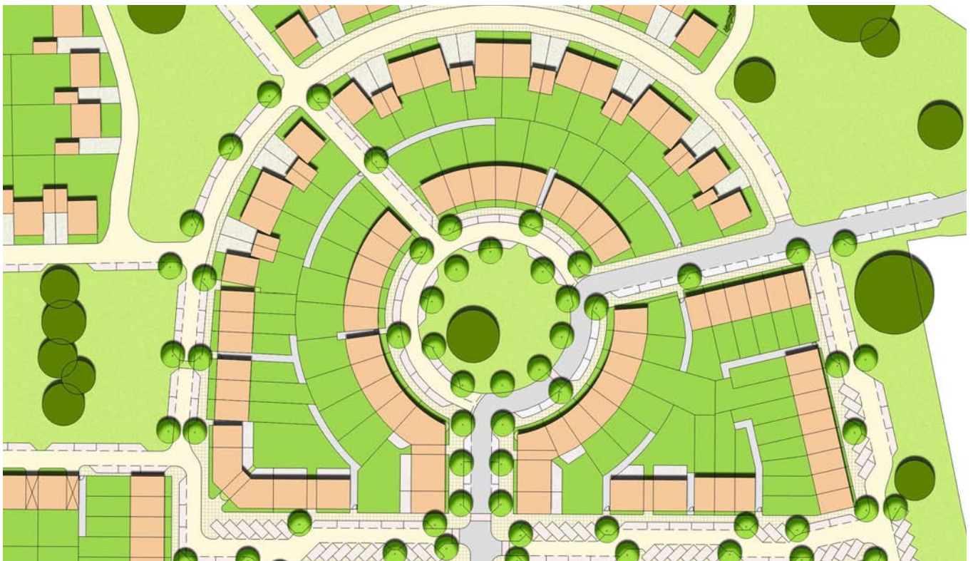
Figure 5.11 This plan suggests how parking may be successfully assimilated into a circus without detriment to the setting of the buildings or the green space.
