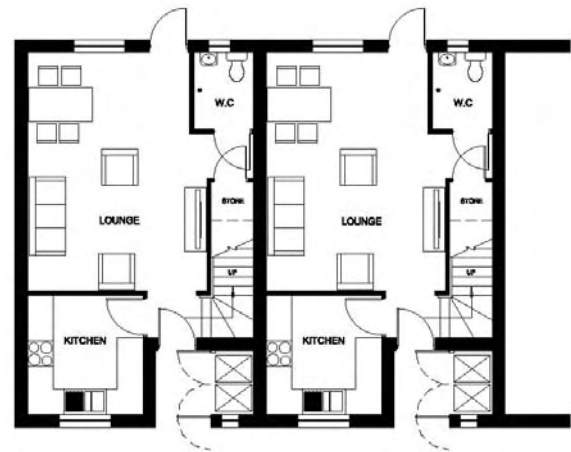
Figure 8.5 Bins are accommodated within footprint of houses
