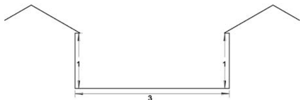
Figure 5.18a This arrangement of two storey houses produces a height to width ratio of 1:3 but the enclosure and townscape is likely to be poor.
