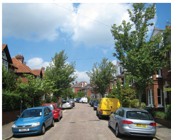
Figure 6.11 A typical terraced street with on-street parking as the main parking provision supplemented by frontage access on-plot parking.
