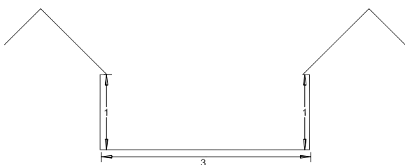
Figure 5.18b The sense of enclosure and quality of the street will be enhanced by steeper pitched roofs.
