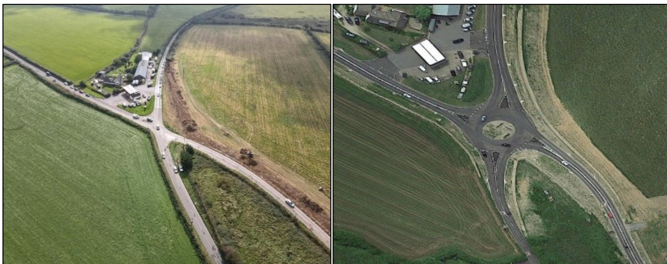
Figure 25: Lynton Cross safety improvements, with crossroads upgraded to a roundabout
