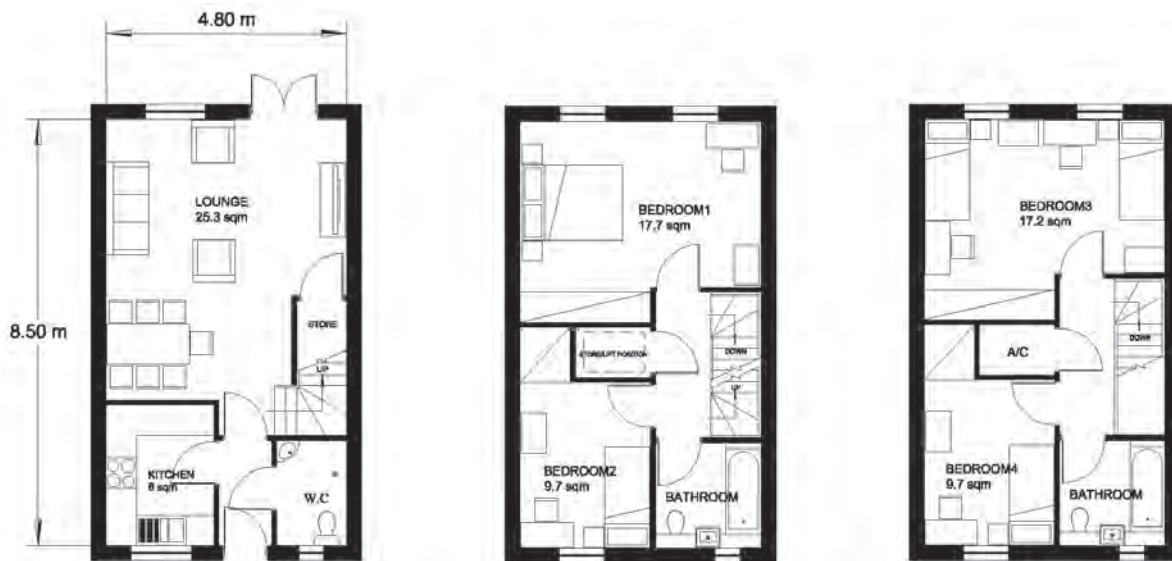
Figure 9.10 An example of 4 bedroom townhouse which meets the standards, Gross Internal Floor Area 117.6 sq metres. Note the increase of the building width by 0.5m and the re-arrangement of the W.C and bathrooms positions help to achieve the required standards.
