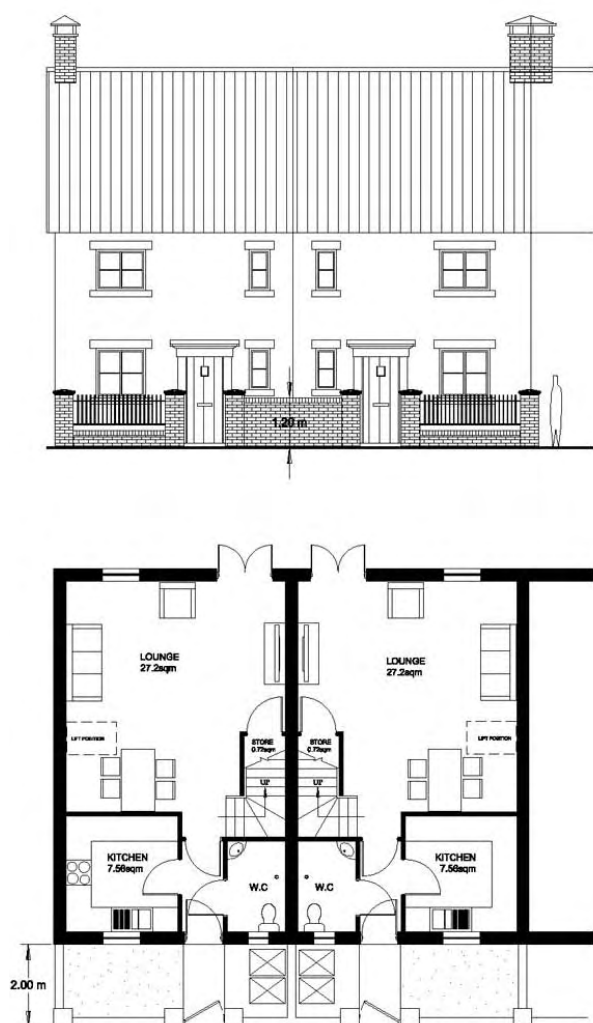
Figure 8.6 Bin store within front gardens
